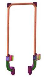
Fig. 4. Finite element model of the ROPS.
