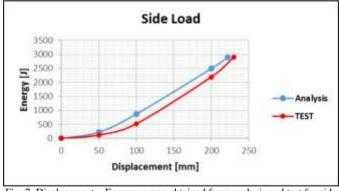
Fig. 7. Displacement - Energy curves obtained from analysis and test for side loading
