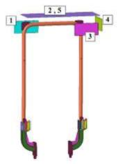
Fig. 2. ROPS loading sequence.
