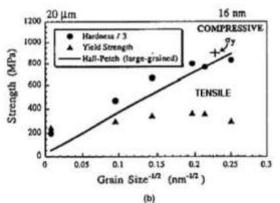
Fig. (b). Positive Hall Petch slope with higher values for compressive than for tensile strength.
