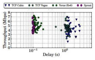
Fig. 4. LTE Throughput vs Delay.
