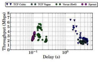
Fig. 3. 3G throughput vs Delay.
