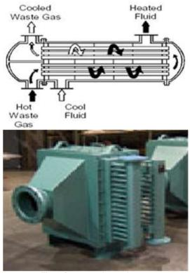
Fig. 5. Gas to water heat exchanger.
