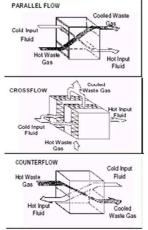
Fig. 4. Sketch for three types of heat exchanger.
