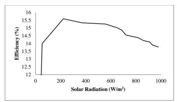
Fig. 7. PV efficiency variation with solar radiation.
