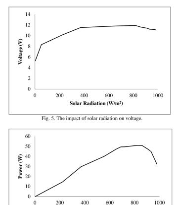
Fig. 6. Solar radiation impact on the generated power.
