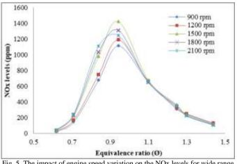
Fig. 5. The impact of engine speed variation on the NOx levels for wide range of equivalence ratio.
