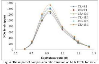
Fig. 4. The impact of compression ratio variation on NOx levels for wid range of equivalence ratios.
