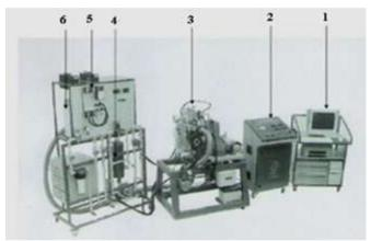
Computer and its accessories 2. Control panel 3. The engine 4. Engine's cooling unit 5. The engine's fuel unit 6. The air supply system Fig. 1. The system used in experiments.
