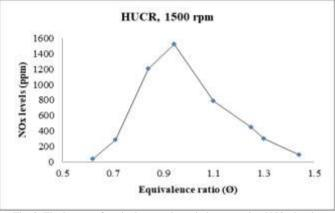
Fig. 2. The impact of equivalence ratio variation on emitted NOx levels.
