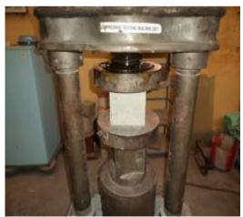
Fig. 4. Cube compression test.
