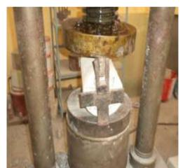
Fig. 5. Split tensile strength.
