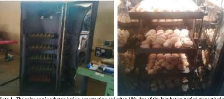
Plate 1. The solar egg incubator during construction and after 18th day of the Incubation period respectively.
