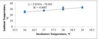
Fig. 2. The regression line and correlation between the interior and ambient temperature of the egg incubator.
