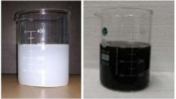
Fig. 3. Al<sub>2</sub>O<sub>3</sub>-water and CuO-water nano-fluid (0.05%) [4]
