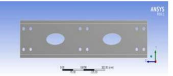
Fig. 6. Lipped channel beams with elliptical opening.
