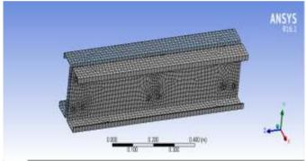
Fig. 3. Meshed view of beam.
