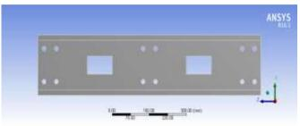
Fig. 4. Lipped channel beams with rectangular opening.
