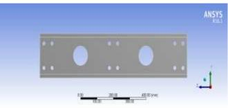
Fig. 5. Lipped channel beams with circular opening.
