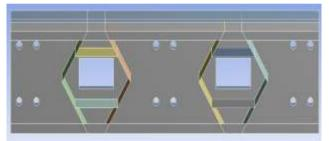
Fig. 9. Rectangular opening with stiffener arrangement 3.
