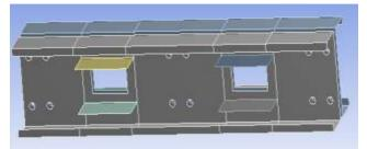
Fig. 8. Rectangular opening with stiffener arrangement 2.
