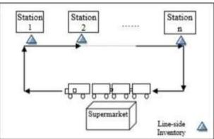
Fig. 1. In-plant milkrun model. [6]
