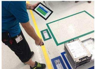
Fig. 3. Recording material flow by scanning QR code. [4]
