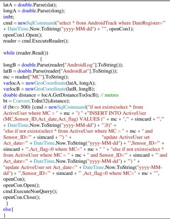
Fig. 5.10. The C# code for determine the radios of the circle around active sensor by 500 Meters.
