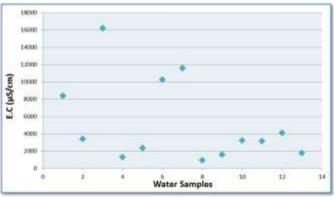
Fig. 5. Salinity index for groundwater samples for Wadi Fatimah area.
