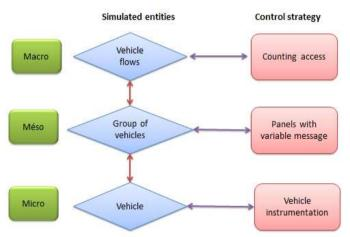
Fig 1. Simulation and hybrid control of traffic flows.
