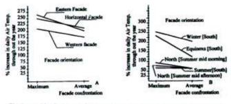
Fig. 5. A and B Maximum and average % increase to the registered air temperatures.
