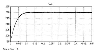
Fig. 14. The Vdc (volt) wave form for three phase PWM rectifier.
