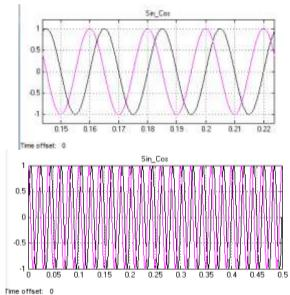
Fig. 13. The sin\_cos wave form for three phase PWM rectifier.
