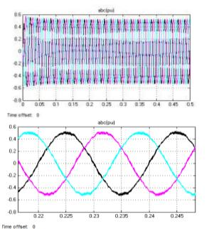
Fig. 10. The abc(pu) wave form for three phase PWM rectifier with controller.
