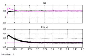
Fig. 9. The Isd & IdIq\_ref wave form for three phase PWM rectifier.
