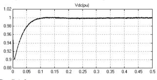
Fig. 15. The Vdc (pu) wave form for three phase PWM rectifier.
