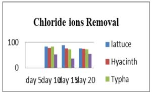
Fig. 6. Chloride reduction with planted and unplanted wetland systems with increasing treatment periods.
