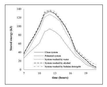
Fig. 4. The stored energy in the target for the studied cases distributed with time
