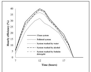
Fig. 5. The hourly efficiency distribution during the day for the studied systems
