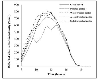
Fig. 2. The reflected solar radiation intensity from mirrors for the studied periods
