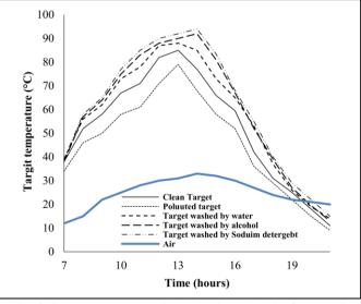
Fig. 3. The target temperature distribution through the day for the studied cases
