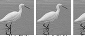
(e) I=15, MSE=26.5 (f) I=20, MSE=25 (d) I=10, MSE=27.1 Fig. 9. Resulted restored Bird image for  $\sigma_e$ =2 for different values of number of iterations applied on degraded image of  $\sigma$ =2 and SNR=30.
