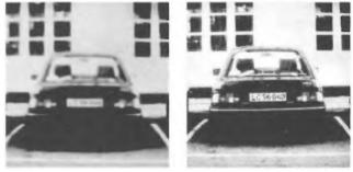
(a) Degraded image. (b) Retrieved image. Fig. 1. Image retrieval by Mead's filter.
