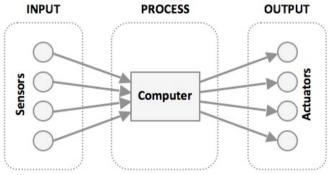
Fig. 1. Basics of computer controlled industrial automation [1].
