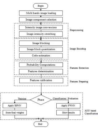
Fig. 2. Block diagram of the proposed satellite image classification.
