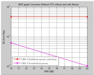
Fig. 10. Graph of BER vs SNR without and with correction moose methods.
