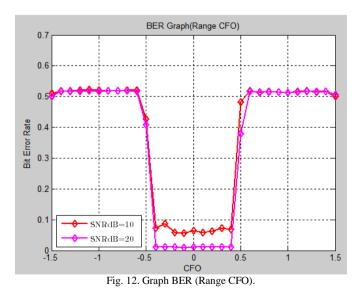
Moose technique when SNR 10dB can better correct the CFO 0.3 while at 20dB moose can correct better the CFO 0.2
