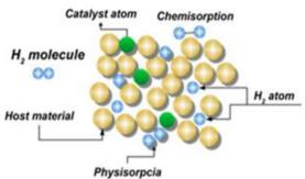
Fig. 1. Chemisorption and physisorption in catalytic materials.
