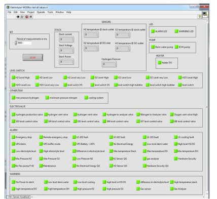
Fig. 12. Visualization of hydrogen accumulation system in the environment of LabView for electrolyzer.
