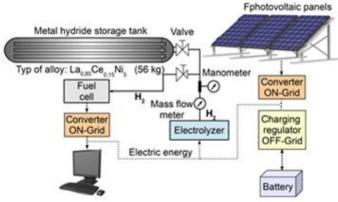
Fig. 1. The solar energy accumulation system using hydrogen technology.
