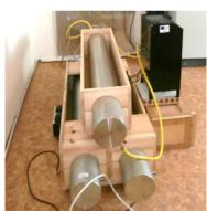
Fig. 7. HBond©9000 metal hydride vessels.
