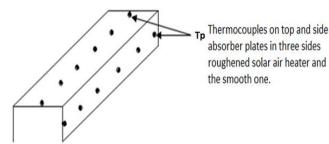
Fig. 3(b.) Thermocouple arrangement on top and sides of three sides roughened and smooth ducts.
