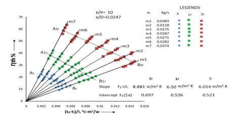
Fig.4. Performance characteristic of solar air heaters
