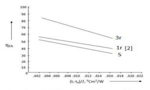
Fig. 7 Thermal efficiency curves for solar air heaters
