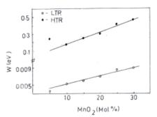
Fig. 6. Variation of activation energy (w) with  $MnO_2$  mol% in LTR and HTR for the glass samples.
