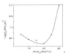
Fig. 7. Variation of pre-exponential factor  $(-\log \sigma_0)$  versus Composition for the glass samples.
