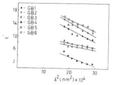
Fig. 3. Plot of optical dielectric constant  $\epsilon$ ' verses  $\lambda$ <sup>'2</sup> for six samples GB<sub>1</sub>, GB<sub>2</sub>, GB<sub>3</sub>, GB<sub>4</sub>, GB<sub>5</sub>, GB<sub>6</sub>.
