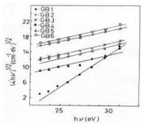
Fig. 2 . Plot of  $\alpha$  'hv verses hv for samples GB<sub>1</sub>, GB<sub>2</sub>, GB<sub>3</sub>, GB<sub>4</sub>, GB<sub>5</sub>, GB<sub>6</sub>.
