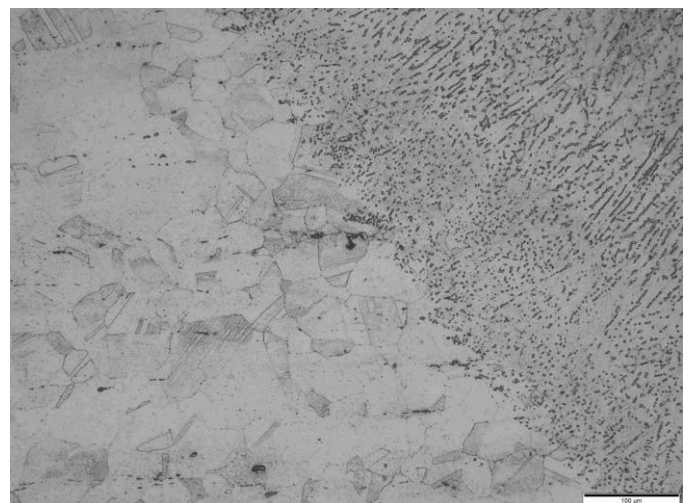
Fig. 12. Interface of Base metal 347& weld metal ER347, 200x.
