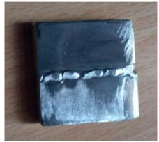
Fig. 9. TIG welded specimen for microscopic analysis.
