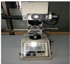
Fig. 6. Vickers hardness test machine.
