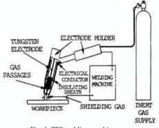
Fig. 1. TIG welding machine setup.
