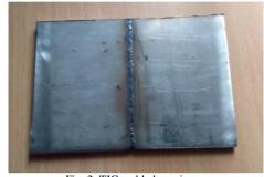
Fig. 2. TIG welded specimen.
