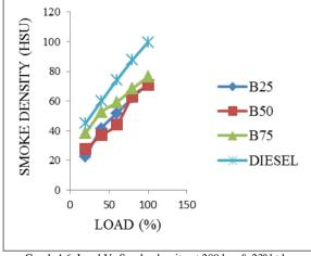
Graph 4.6. Load V<sub>s</sub> Smoke density at 200 bar & 23° btdc.
