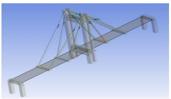
Fig. 5. Straight cable stayed bridge with H shape pylon.
