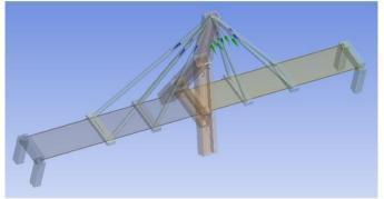
Fig. 6. Straight cable stayed bridge with inverted Y shape pylon
