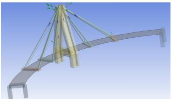
Fig. 1. Curved cable stayed bridge with A shape pylon.
