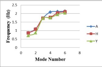
Fig. 9. Variation of modal frequency with mode number for straight bridge systems.
