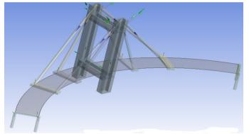
Fig. 2. Curved cable stayed bridge with H shape pylon.
