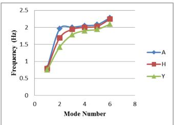
Fig. 8. Variation of modal frequency with mode number for curved bridge systems.
