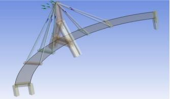
Fig. 3. Curved cable stayed bridge with inverted Y shape pylon.
