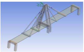
Fig. 4. Straight cable stayed bridge with A shape pylon.
