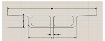
Fig. 7. Cross-sectional details circular straight box girder (all dimensions are in meter).
