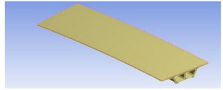
Fig. 6. Perspective view of trapezoidal curved box girder.
