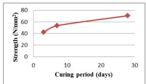
Fig. 1.Graphical representation of compressive strength of control mix.
