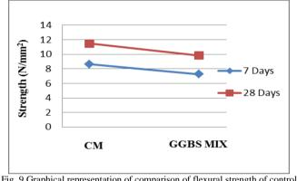
Fig. 9.Graphical representation of comparison of flexural strength of control mix and GGBS mix.
