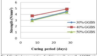
Fig. 5.Graphical representation of splitting tensile strength of GGBS mix.
