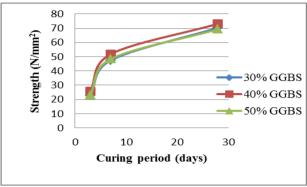
Fig. 4.Graphical representation of compressive strength of GGBS mix.
