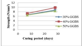
Fig. 6.Graphical representation of flexural strength of GGBS mix.
