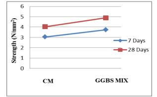
Fig. 8.Graphical representation of comparison of splitting tensile strength of control mix and GGBS mix.
