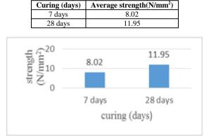
Fig. 6. Graphical representation of flexural strength of optimum percentage of metakaolin.
