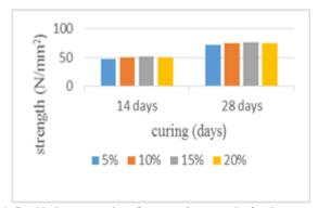
Fig. 4. Graphical representation of compressive strength of various percentage of metakaolin.
