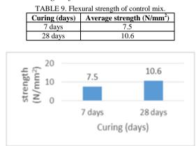
Fig. 3. Graphical representation of flexural strength of control mix.
