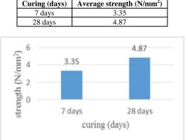
Fig. 5. Graphical representation of split tensile strength of optimum percentage of metakaolin.
