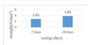
Fig. 2. Graphical representation of split tensile strength of control mix.
