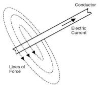
Fig. 4. Principle of electro magnet.
