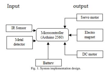
The above figure 1 describes the system implementation design where Arduino is the heart of the system because it controls the both input and output.
