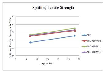
Fig. 6.Graphical representation of split tensile strength of SCC and SCC with Optimum Alccofine and Micro steel fiber.
