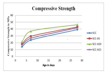
Fig. 2. Graphical representation of compressive strength of SCC and SCC with Alccofine.
