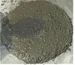
Fig. 1. Slump flow.
