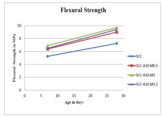
Fig. 7.Graphical representation of flexural strength of SCC and SCC with Optimum Alccofine and micro steel fiber.
