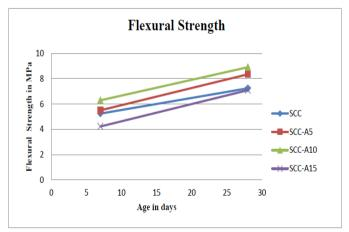
Fig. 3.Graphical representation of flexural strength of SCC and SCC with Alccofine.
