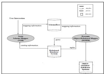
Fig. 1. Overall system architecture.
