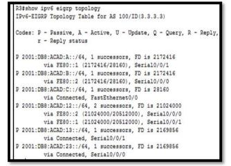
Fig. 7. shows topology table of router R3.
