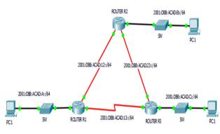
Fig. 1. Implemented topology in packet tracer.
