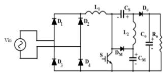
Fig. 3. Modified SEPIC Converter.
