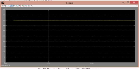
Fig. 10. Output voltage of the modified SEPIC converter.
