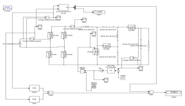
Fig. 9. Matlab simulation of the modified SEPIC converter wth third harmonic reduction technique.
