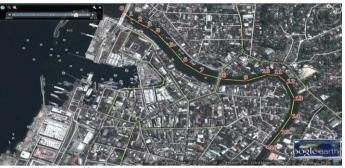
Fig. 1. Position of point measurements and model boundaries Along the Tondano estuary.
