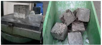
Fig. 2. Compressive Strength Test (a) While testing (b) Crushed cubes.
