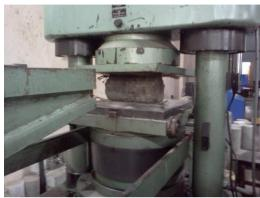
Fig. 4. Splitting tensile strength test.
