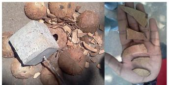
Fig. 1. Crushed coconut shells.
