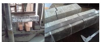
Fig. 3. Flexure Strength Test (a) While testing (b) After testing.
