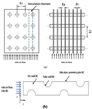
Modelled heat exchanger: (a) nomenclature and simulation domain. (b) Computational domain with boundary conditions.
