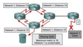
Fig. 2. Count to infinity that limits RIP network diameter of 15 or fewer hops.
