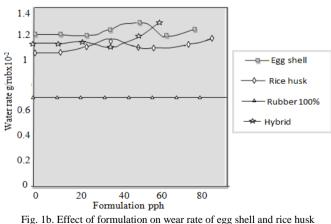
Fig. 1b. Effect of formulation on wear rate of egg shell and rice husk composites.
