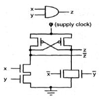
So by substituting the value of y and at the positions of F and F/ n tree positions in the figure 1 respectively we get the AND circuit implementation using ECRL technology.
