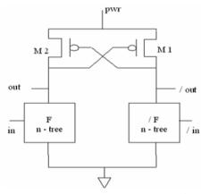
Fig. 3. Efficient charge recovery logic (ECRL)
