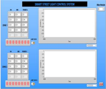
Fig. 2. Front panel of smart street light.
