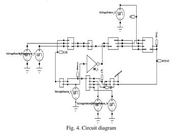
It is the circuit diagram of the proposed methodology, where the circuits designed for the Adaptive Hold Logic are converted into symbols. And it is called back to the design at the time of simulating. The input bits are given through voltage source
