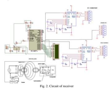
The patients, medical staffs etc. uses RFID TAG. An inductively coupled transponder comprises of an electronic data-carrying device, usually a single microchip and a large area coil that functions as an antenna. Inductively coupled
