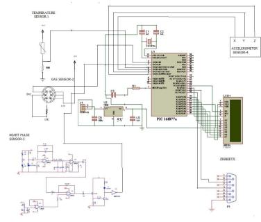
Fig. 1. Circuit of transmitter
