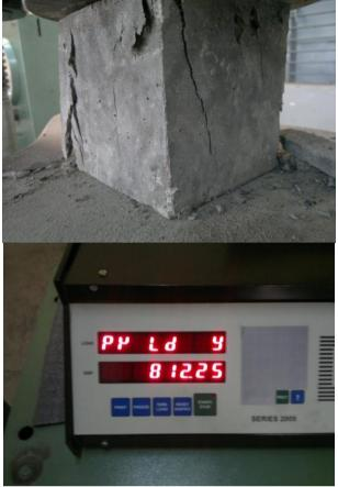
Fig. 2. Testing of cube in CTM
