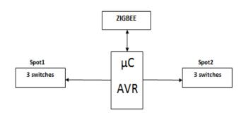
Recommended schematic of the plant node
