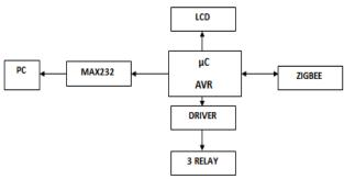
Recommended schematic of the warehouse node
