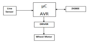
Recommended schematic of the locomotive vehicle
