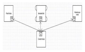
Recommended schematic of the object- handling system
