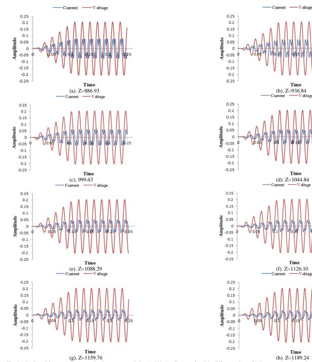
Fig. 1(a-h). Signal for output current and voltage are recorded at 16,000 sampling rate for eight different values of inductance, keeping resistance (36Ω) and capacitor are constant.
