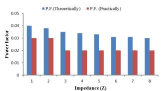
Fig. 3. Theoretical and practical calculated value of power factor for different combinations of impedance (LC with resistor 36  $\Omega$ ).
