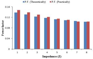
Fig. 4. Calculated the theoretical and practical value of power factor for certain combinations of impedance (LC with resistor 124  $\Omega$ ).
